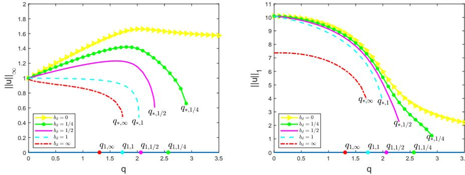
FIG. 8. Comparison of bifurcation points  $q_1$ ,  $q_*$ , and maximal steady state solutions of (2.1) under different boundary conditions. Here  $g(x, u) = (r - u)(u + h)$ ,  $r = 1$ ,  $h = 0.3$ ,  $b_u = 0$  (NF boundary condition on the upstream end),  $d = 4$ ,  $L = 10$ , and the horizontal axis is  $q$ . Left: comparison of  $\|u\|_\infty$ . Right: comparison of  $\|u\|_1$ .
