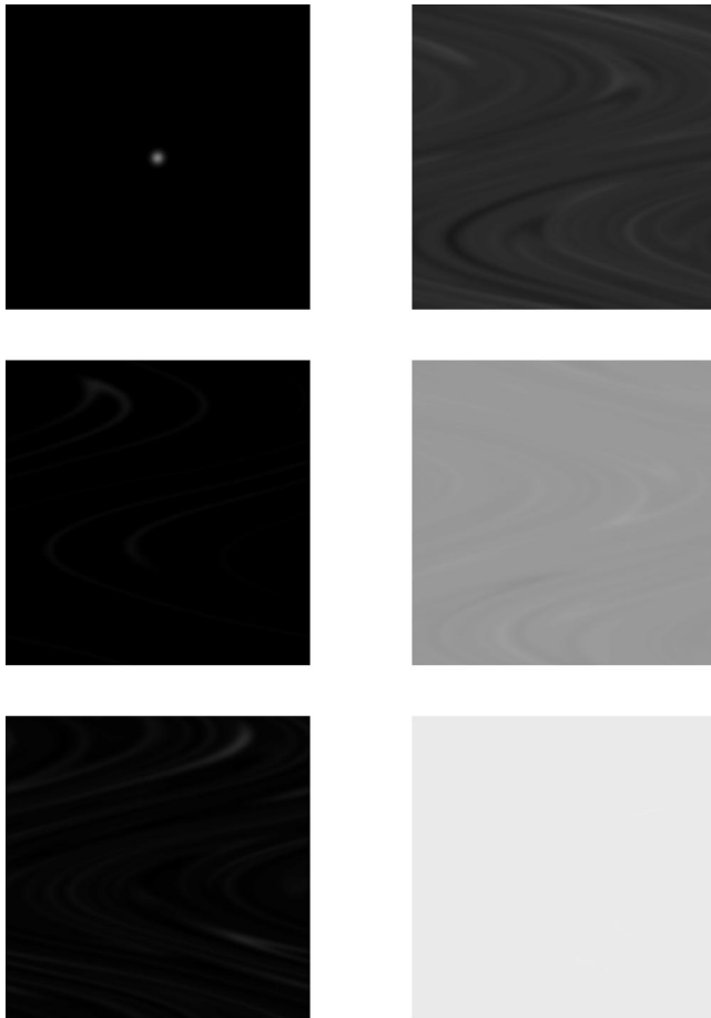
FIG. 1. Snapshots of the spatial distribution for the autocatalytic reaction for Da=1.0 (<Da_c) at t=0.0, 2.0, 4.0, 6.0, 8.0 . The amplitude of the initial perturbation is chosen to be C_0=0.5 in order to make the initial decay visible.
