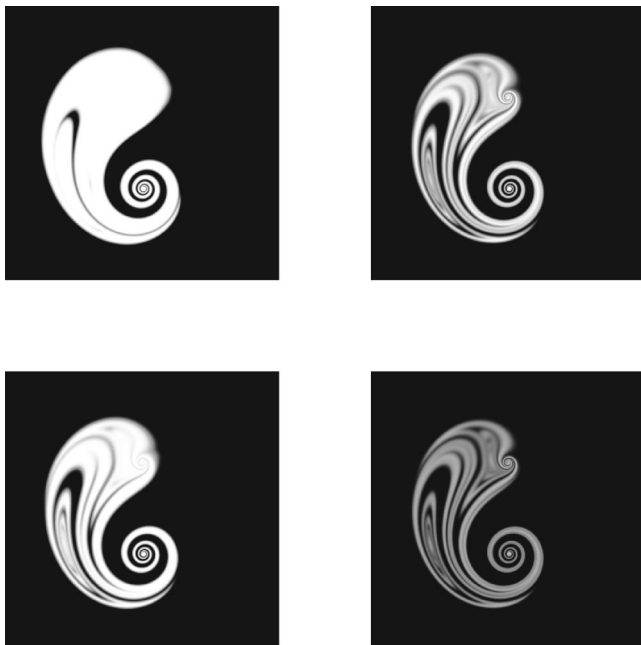
FIG. 7. Snapshots of the spatial distribution for the autocatalytic reaction in the open flow system for a supercritical Damköhler number, Da=14.0 > Da_c at t=0.0, 1.0, 2.0, 3.0, 4.0, 5.0 . The distribution at t=5.0 has already reached the time-periodic stationary state. The amplitude of the perturbation is C_0=0.5 . For subcritical Damköhler numbers the perturbation dies out. (The bistable model shows similar behavior but for different values of Da .)
